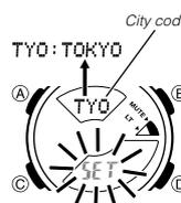
1. In the Timekeeping Mode, hold down (A) for about two seconds until "SET" appears on the lower display. This is the setting mode.
