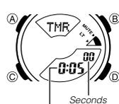
You can set the countdown timer start time within a range of one minute to 24 hours. An alarm sounds when the countdown reaches zero.
