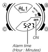
When an alarm is turned on, the alarm tone will sound when its alarm time is reached. One of the alarms is a snooze alarm, while the other four are daily alarms. You also can turn on an Hourly Time Signal that causes the watch to beep twice every hour on the hour.
